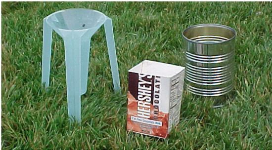
Suitable test containers could include special water measuring cups, open-topped milk cartons, or soup cans.
